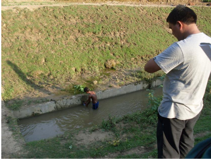
Measurement of water discharge at point source from Ramjanaki forest into irrigation canal
